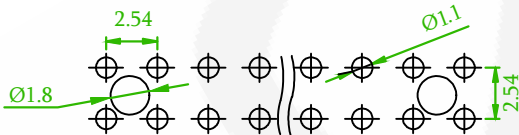
RECOMMENDED PCB LAYOUT (PCB TOLERANCE ±0.05)
