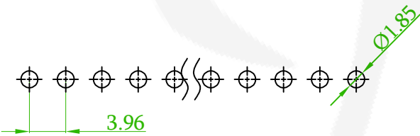
Recommended PCB Layout (PCB TOLERANCE ±0.05)
