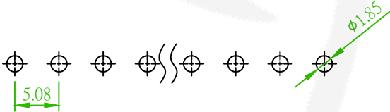
Recommended PCB Layout (PCB TOLERANCE ±0.05)
