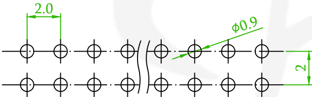
Recommended PCB Layout (PCB TOLERANCE ±0.1)
