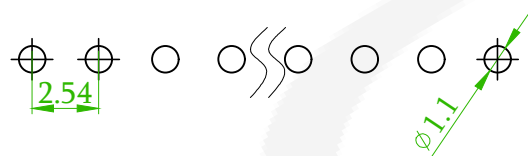
Recommended PCB Layout (PCB TOLERANCE ±0.1)
