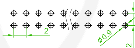
Recommended PCB Layout (PCB TOLERANCE ±0.1)
