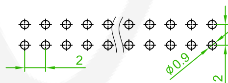
Recommended PCB Layout (PCB TOLERANCE ±0.1)
