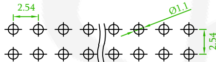
Recommended PCB Layout (PCB TOLERANCE ±0.1)
